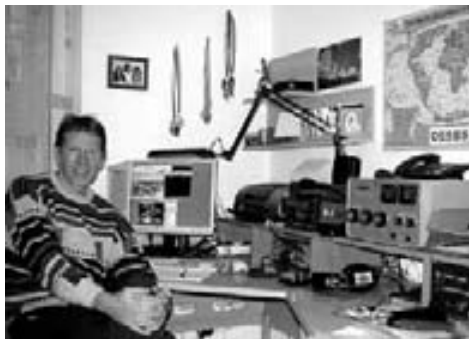
2005: TS-570D, IC-751, TS-711, Longwire 20 m, GP 2 Meter.
